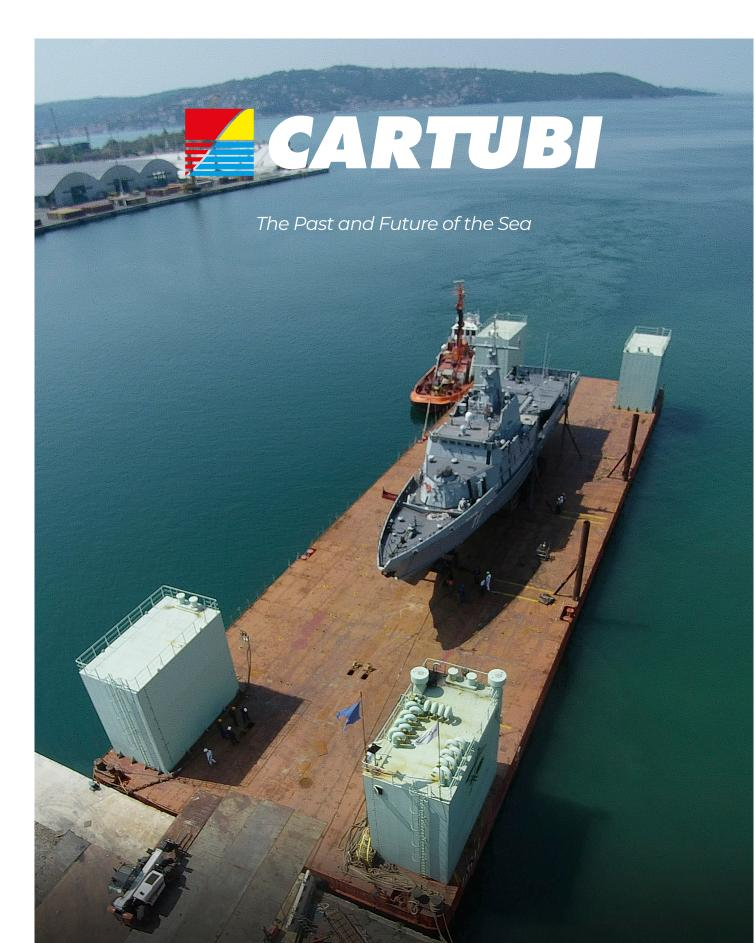
Semi-submersible Heavy Lift Barge
